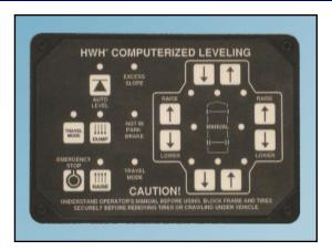
● Our system features computer (touchpanel) control and our HWH® L e v e l e z e ® Indicator Light System. The control pad can be dash mounted for operator convenience.
