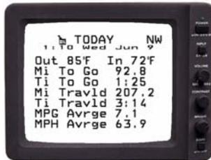
Press the **VIEW** key on the keypad. The “TODAY” screen will display on the backup monitor.
