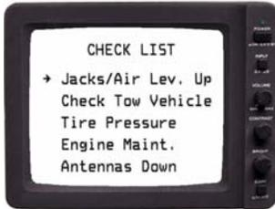
With the above steps completed, the “CHECK LIST” screen will be displayed on the backup monitor.
