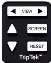
Press the up  $\Delta$  or down  $\nabla$  key to step through each line item to choose the appropriate screen.
