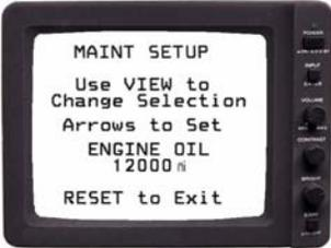
**Engine Oil:** Selected maintenance item to set. Ref. Engine Oil, Eng. Fuel Filter, Transmission Oil, Generator Oil and Fuel Filter
