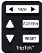
If a line item is blinking, press **VIEW**  $\blacktriangleright$  to move to the appropriate screen (i.e. “MAINTENANCE”) to evaluate the problem.
