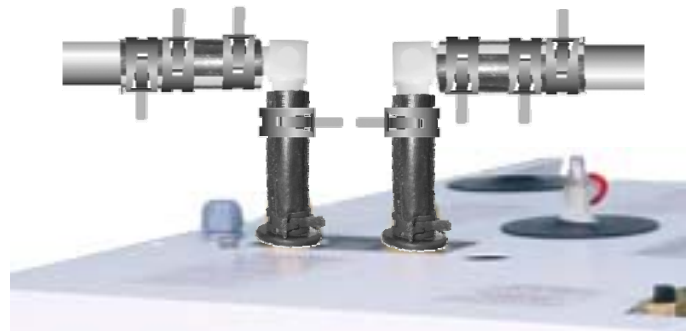
90° Connection Components Installed
